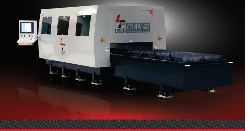
Using a new high performance, energy-efficient fiber laser, this system will achieve a level of quality and detail that is unprecedented in the industry for laser cutting. It can cut aluminum, anodized aluminum, alloy metals, stainless steel, mild steel, copper, brass, non transparent plastics, plaques, create stencils, and more.
