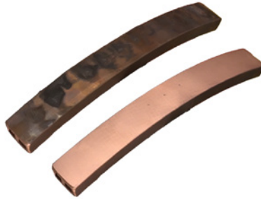
Corrosion Removal on Brass
