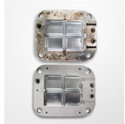
Corrosion Removal on Aluminum Mold
