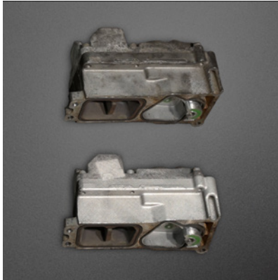
Corrosion Removal on Aluminum Housing
