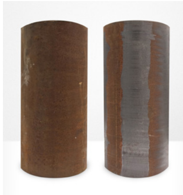
Corrosion Removal on Steel Cylinder
