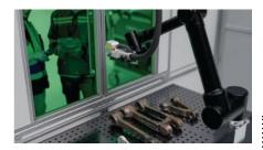
By integrating lasers with advanced robotics within enclosed workcells, this technology allows for efficient, repeatable cleaning of components of various sizes.
