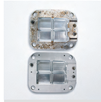
Corrosion Removal on Aluminum Mold
