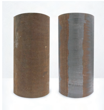
Rust Removal on Steel Cylinder
