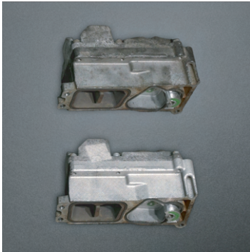
Corrosion Removal on Steel Housing
