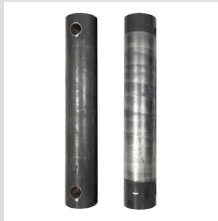
Laser Cleaning on Steel Pipe
