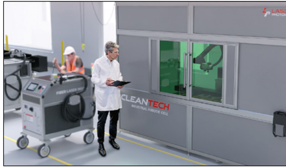
Robotic work cells, equipped with laser-welding robots and safety features, enable repetitive tasks like laser cleaning to be automated, freeing employees for other tasks. (Image: Laser Photonics)
