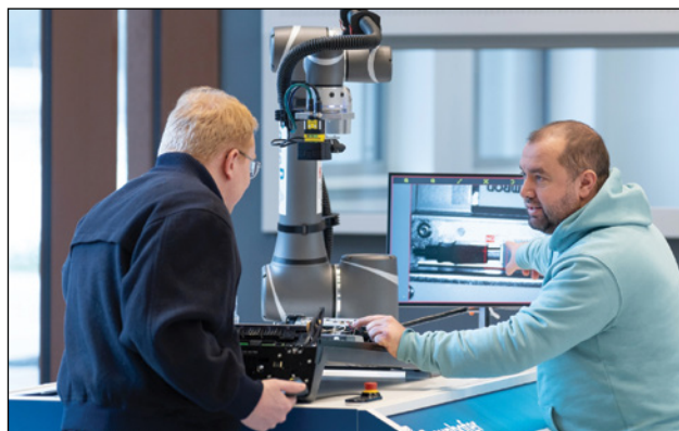
Collaborative robots free production employees from having to perform labor-intensive and error-prone manual visual inspections. (Image: Fraunhofer Institute for Mechatronic Systems Design)
