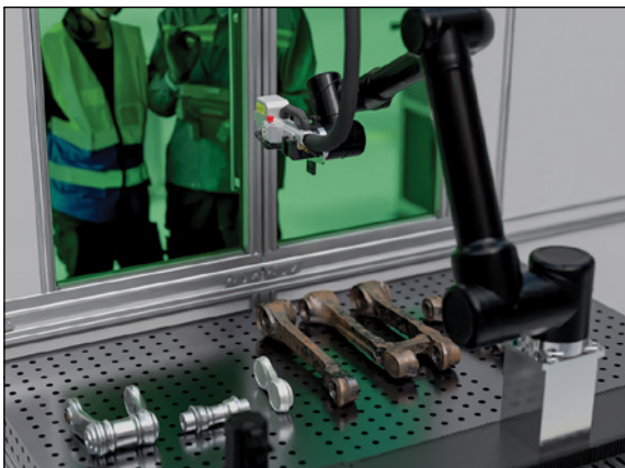
By integrating lasers with advanced robotics within enclosed work cells, this technology allows for efficient, repeatable cleaning of components of various sizes. (Image: Laser Photonics)
